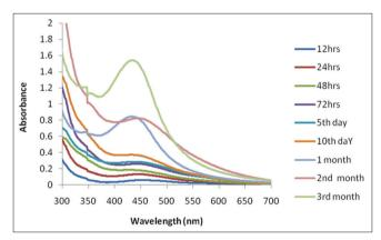
Fig. 5: Ultraviolet-visible spectrum of the silver nanoparticles at different time durations
