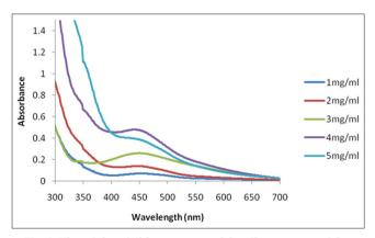
Fig. 1: Ultraviolet-visible spectrum of the silver nanoparticles synthesized using a different concentration of plant extract
