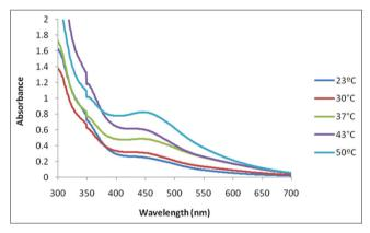
Fig. 2: Ultraviolet-visible spectrum of the silver nanoparticles synthesized at the different reaction temperature
