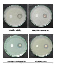
Fig. 9: Antibacterial activity of the cotton fabric incorporated with silver nanoparticles
