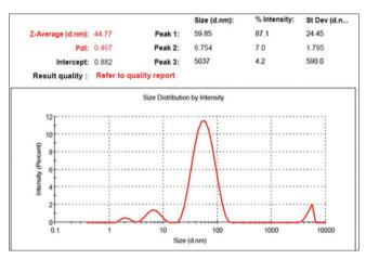
Fig. 7: Dynamic light scattering analysis of synthesized silver nanoparticles
