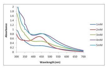
Fig. 4: Ultraviolet-visible spectrum of the silver nanoparticles synthesized at different concentration of silver nitrate
