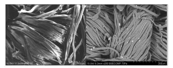
Fig. 10: Scanning electron microscope analysis of untreated and cotton fabric incorporated with silver nanoparticles
