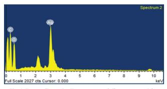
Fig. 4: Energy dispersive X-ray spectra of silver nanoparticles
