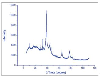
Fig. 5: Energy dispersive X-ray pattern of silver nanoparticles synthesized using extract of *Ipomoea batatas*
