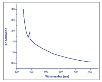
Fig. 2: Ultraviolet-visible spectra of silver nanoparticles synthesized using extract of *Ipomoea batatas*
