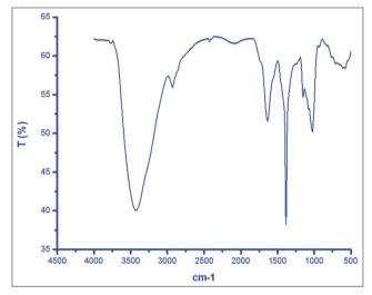
Fig. 1: Fourier-transform infrared spectroscopy spectra of silver nanoparticles synthesized using extract of *Ipomoea batatas*
