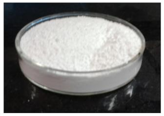
Fig. 1: Silver-doped hydroxyapatite in powder form
