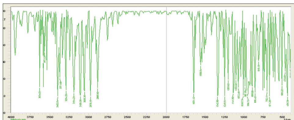
Fig. 2: Fourier-transform infrared spectrum of meloxicam
