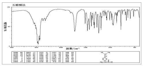
Fig. 1: Fourier transform infrared pure ibuprofen
