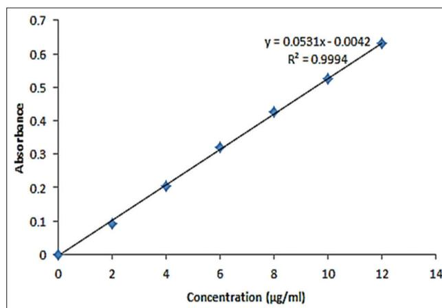
Fig. 1: Standard calibration curve of cefixime in methanol:water (70:30) at 254 nm; sample size=6 concentrations (at triplicate runs)
