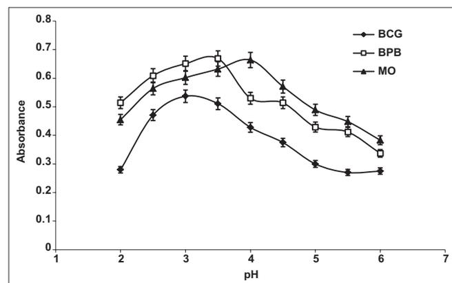
Fig. 2: Effect of pH of buffer solution on the ion-pair complex formation between (10, 12, and 15 µg/ml) MNT and ( $1.0 \times 10^{-3}$  mol/l) bromocresol green, bromophenol blue, and methyl orange reagents, respectively (n=3.0)
