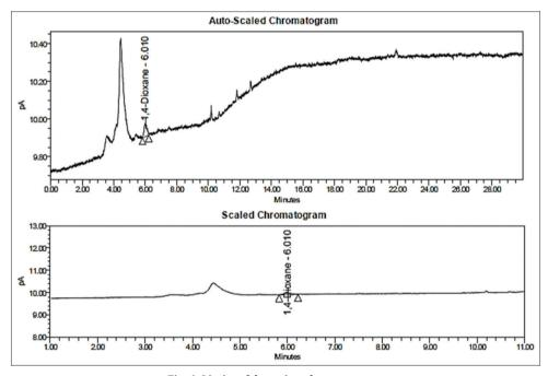
Fig. 6: Limits of detection chromatogram
