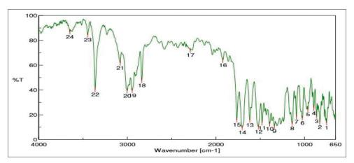
Fig. 5: Fourier-transform infrared spectra of apremilast
