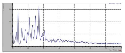
Fig. 4: X-ray diffraction of apremilast cocrystals
