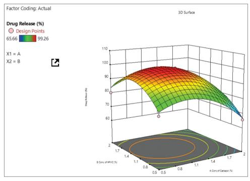
Fig. 10: Three dimensional plot of in vitro drug release
