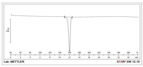
Fig. 1: Differential scanning calorimetry of pure apremilast
