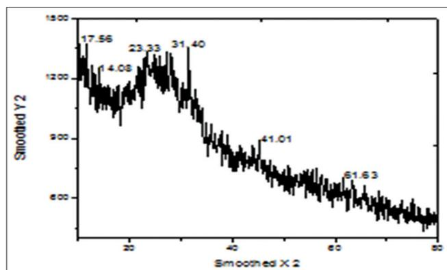
**Fig. 1: X-ray diffraction pattern of iron nanoparticles**
