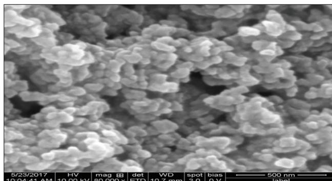
**Fig. 4: Scanning electron microscope image of iron nanoparticles (500 nm views)**
