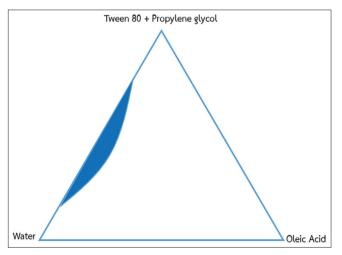
Fig. 3: Pseudoternary phase diagram of microemulsion
