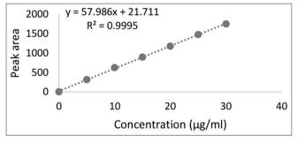
Fig. 4: Linearity curve of Fimasartan
