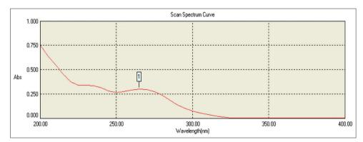
Fig. 2: Ultraviolet spectra of Fimasartan
