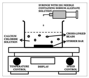
Fig. 2: Schematic illustration of the ionic gelation method. Adapted from reference [30]. Copyright permission obtained under creative commons (CC BY) license. (http:// creativecommons.org/licenses/by/4.0/)
