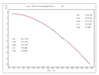
Fig. 13: Differential scanning calorimetry thermogram of Eudragit-S 100
