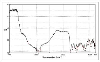
Fig. 2: Fourier transform infrared spectrum of Eudragit- S-100
