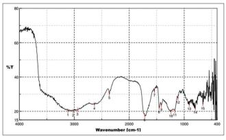
Fig. 3: Fourier transform infrared Spectrum of Carbopol-940
