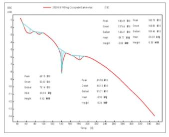
Fig. 12: Differential scanning calorimetry thermogram of ciclopirox olamine
