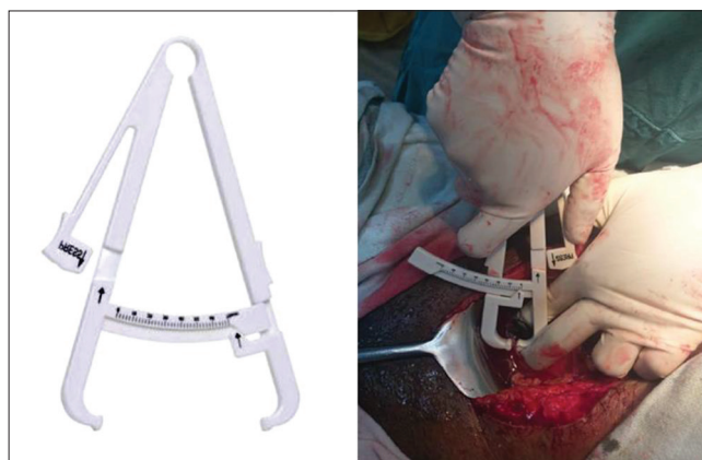
Fig. 2: Caliper used for intraoperative measurements (personal body clip fat measurement tool skinfold test instrument normally used as body fat tester)
