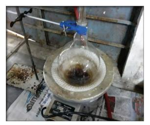
Fig. 2: Extraction using Soxhlet apparatus
