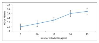
Fig. 4: Standard calibration curve for the polyphenol content using catechol as standard. Conc.: concentration; OD: optical density
