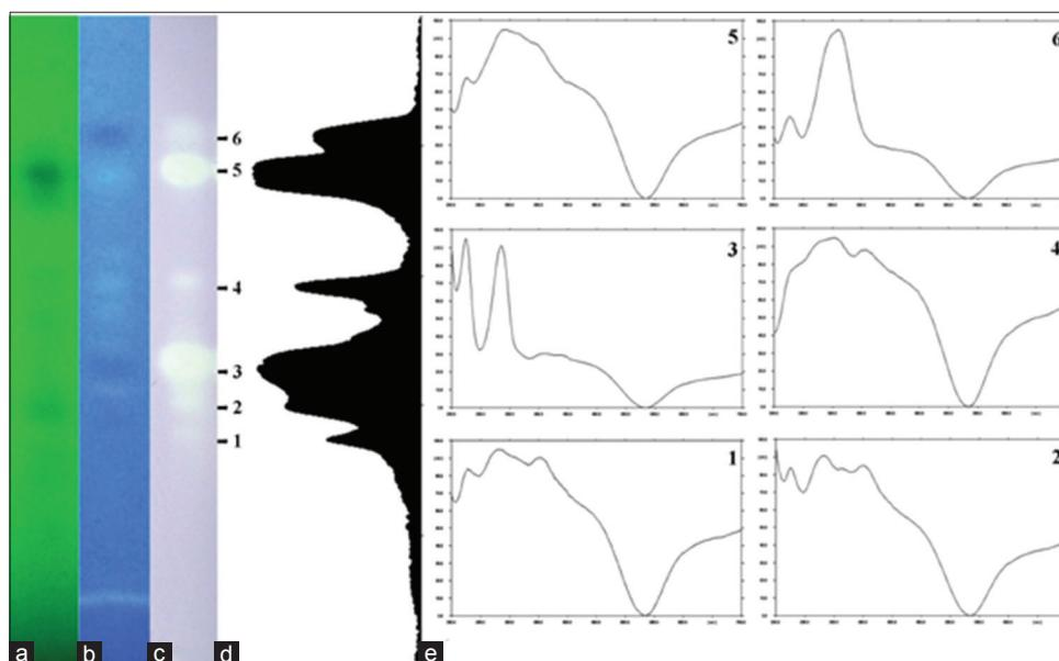
Fig. 4: High performance thin layer chromatography (HPTLC) profile of ethanolic extract of *Bacopa chamaedryoides* after derivatization with 2.54 mM 2,2-diphenyl-1-picrylhydrazyl. (a) Under UV 254 nm; (b) Under UV 366 nm; (c) Under day light and (d) HPTLC densitogram at 600 nm. (e) Absorption spectrum of the six antioxidant bands
