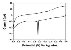
Figure 6: Cyclic voltammograms of silver nanoparticles.
