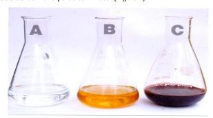
Figure 1: Photographs showing A) pure AgNO<sub>3</sub> solution B) pure *M.Tinctoria* fruit Extract C) Colour changes after adding fruit Extract with AgNO<sub>3</sub> solution.
