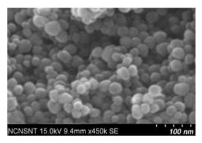
Figure 4: SEM analysis of Silver nanoparticles
