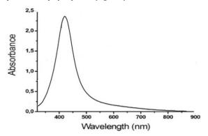
Figure 2: UV Spectra of silver nanoparticles
