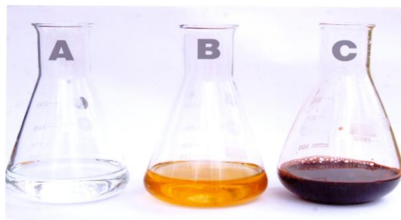
Figure1: Photographs showing A) pure AgNO_3 solution B) pure M.Tinctoria fruit Extract C) Colour changes after adding fruit Extract with AgNO_3 solution.
