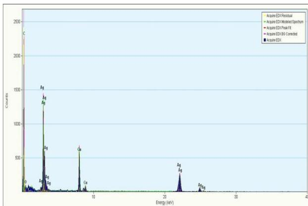
Figure 9: EDAX spectra of Silver Nanoparticles
