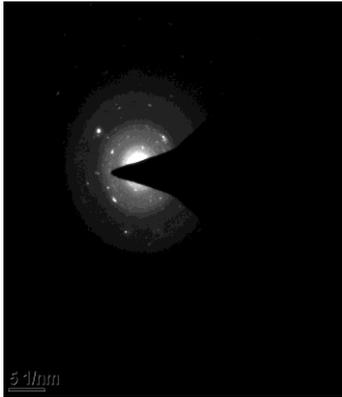
Figure 8c: Selected area Electron Diffraction Pattern (SAED)
