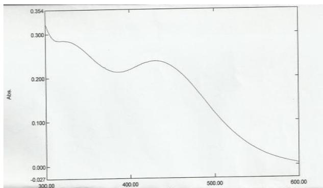
Figure2a : UV-VIS spectrum of Ag nanoparticles under optimum conditions
