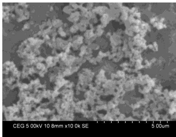
Figure 7: SEM micrograph of Silver Nanoparticles.
