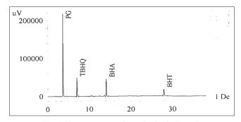
Fig. 1: Chromatogram of standard solution mix
