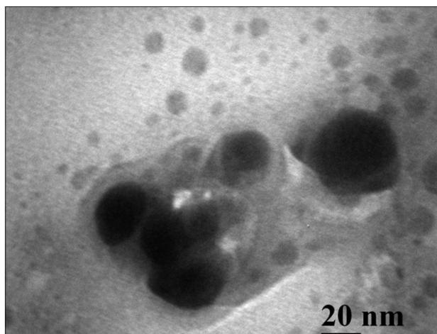
Fig. 5: The transmission electron microscopy image of silver nanoparticles
