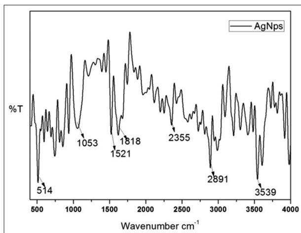
Fig. 2: The Fourier transform infra-red spectrum of isolated silver nanoparticles
