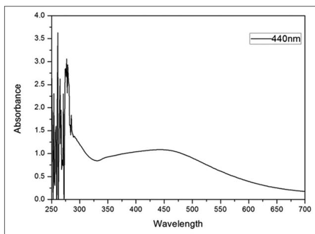
Fig. 1: The ultraviolet-Vis spectrum of silver nanoparticles
