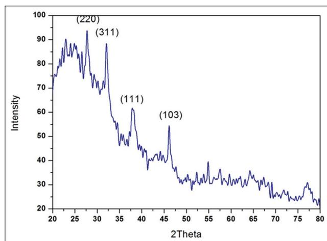
Fig. 3: The X-ray powder diffraction patterns of silver nanoparticles
