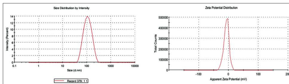
Fig. 4: Hydrodynamic results of silver nanoparticles and surface charge of the silver nanoparticles by DLS.
