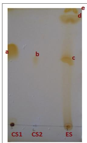
**Fig. 3: Determination of statin from *Aspergillus tamarii* GRD119 in thin layer chromatography. CS1 - 25 µg/ml commercial standard simvastatin (0.625 cm); CS2 - 10 µg/ml commercial standard lovastatin (0.59 cm); ES - Fungal statin (0.59 cm); a, b, c, d - Distance travelled by solute; e - Distance travelled by solvent**
