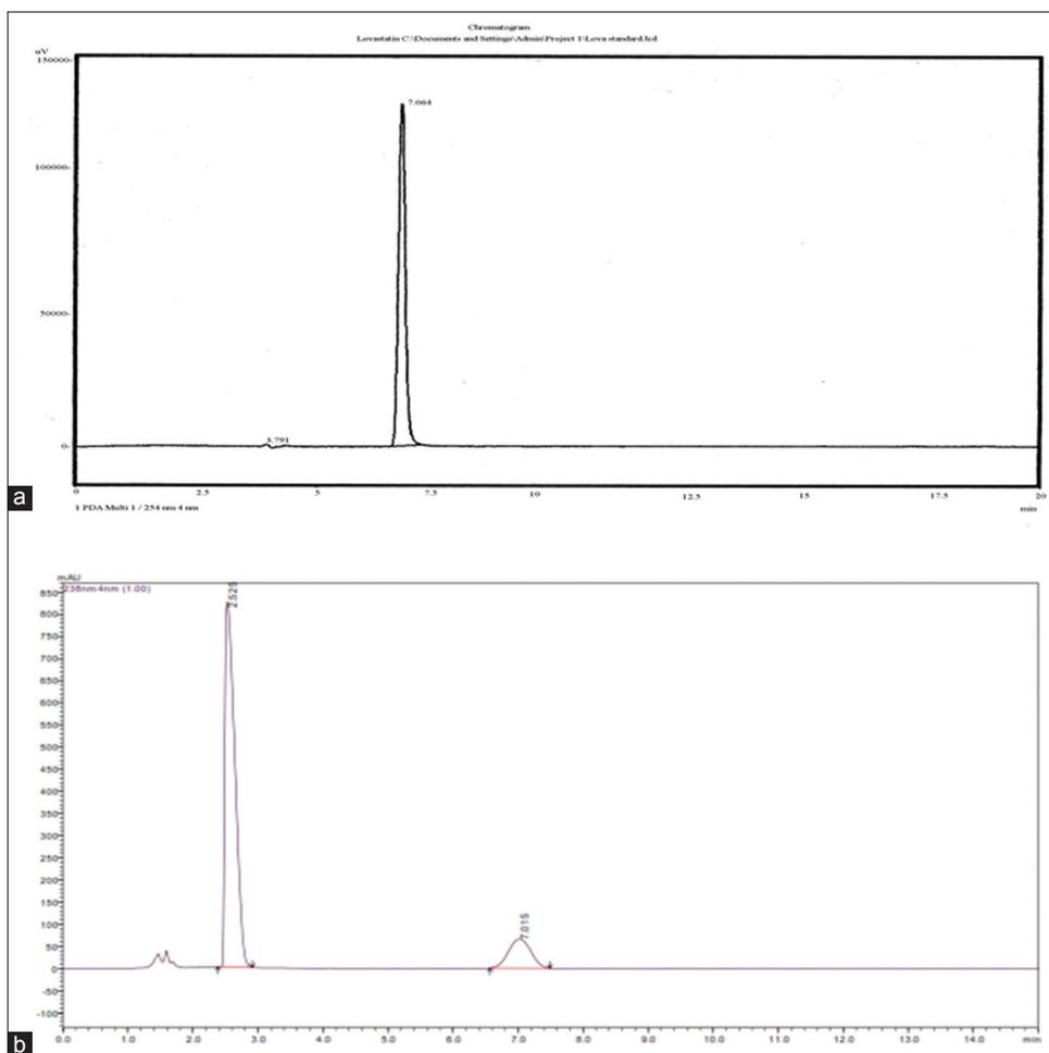
Fig. 5: (a) High-performance liquid chromatography (HPLC) showing the concentration of commercial statin. (b) HPLC Chromatogram showing concentration of crude fungal statin
