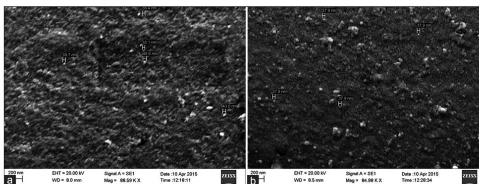
Fig. 3: (a) Scanning electron microscope (SEM) image of silver nanoparticles (SNP's) synthesized from *Simarouba glauca* leaf extract. (b) SEM image of SNP's synthesized from *Artocarpus altilis* leaf extract
