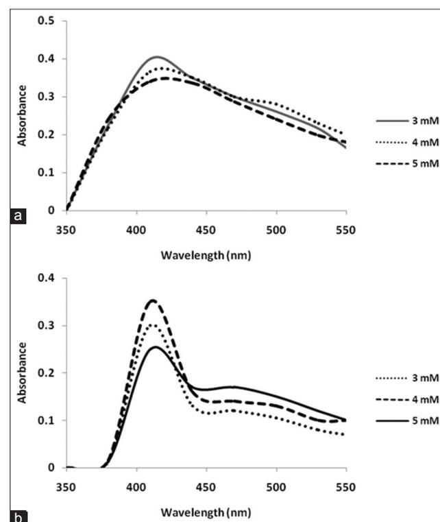
Fig. 2: (a) UV-vis spectra of silver nanoparticles (SNPs) synthesized from *Simarouba glauca* leaf extract recorded as a function of the different concentration of silver nitrate. (b) UV-Vis spectra of SNP's synthesized from *Artocarpus altilis* leaf extract recorded as a function of the different concentration of silver nitrate.
