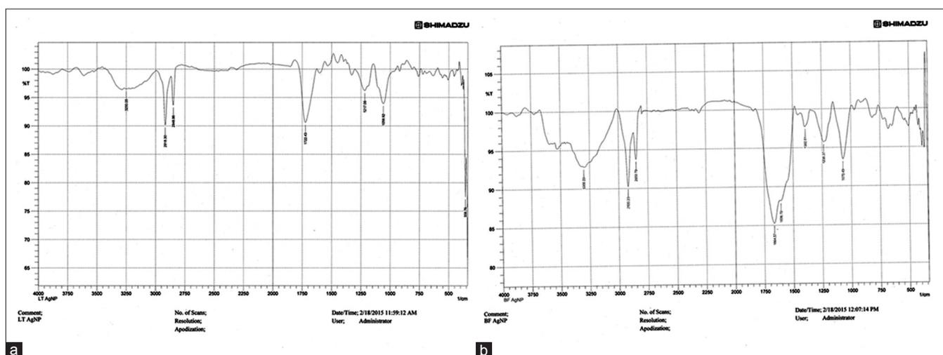
Fig. 4: (a) Fourier transform-infrared spectroscopy (FTIR) spectra of silver nanoparticles (SNP's) synthesized from *Simarouba glauca* leaf extract. (b) FTIR spectra of SNP's synthesized from *Artocarpus altilis* leaf extract
