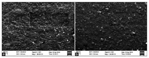
Fig. 3: (a) Scanning electron microscope (SEM) image of silver nanoparticles (SNP's) synthesized from *Simarauba glauca* leaf extract. (b) SEM image of SNP's synthesized from *Artocarpus altilis* leaf extract
