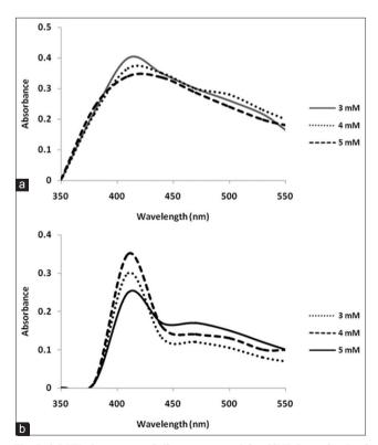
Fig. 2: (a) UV-vis spectra of silver nanoparticles (SNPs) synthesized from Simarauba glauca leaf extract recorded as a function of the different concentration of silver nitrate. (b) UV-Vis spectra of SNP's synthesized from Artocarpus altilis leaf extract recorded as a function of the different concentration of silver nitrate.
