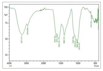
Fig. 1: Fourier transform infrared spectroscopy spectrum of biosynthesized titanium dioxide nanoparticles
