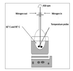
Fig. 4: Liquid-liquid suspension polymerization
