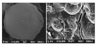
Fig. 1: Typical image of microsponge (a) and its porous surface morphology (b)
