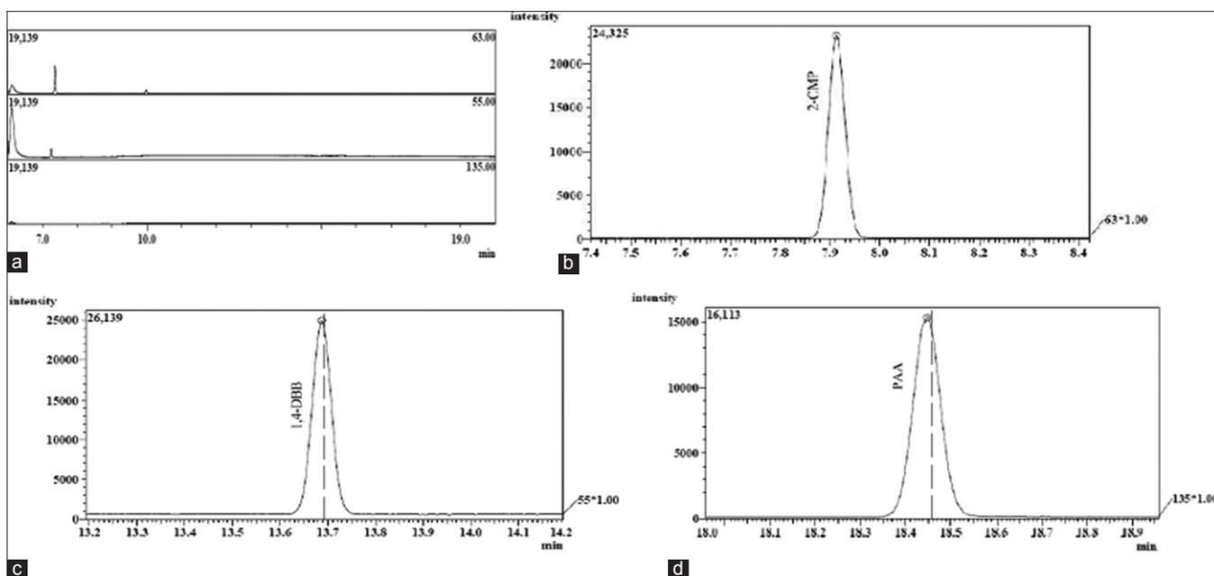
Fig. 4: Specificity chromatograms of (a) blank, (b) 2-chloro methyl propionate, (c) 1,4-dibromo butane, (d) para anisic aldehyde
