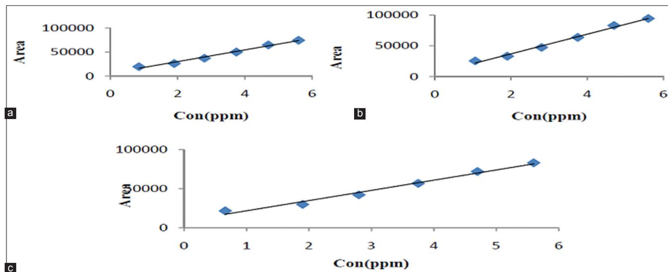
**Fig. 7: Linearity graphs for (a) 2-chloro methyl propionate, (b) 1,4-dibromo butane and (c) para anisic aldehyde at limit of quantification**
