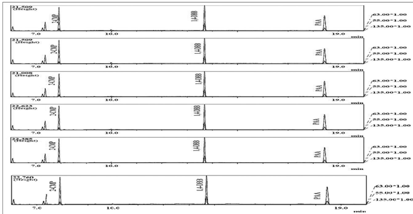
Fig. 5: Typical % relative standard deviation chromatogram of precision for 2-chloro methyl propionate, 1,4-dibromo butane and para anisic aldehyde
