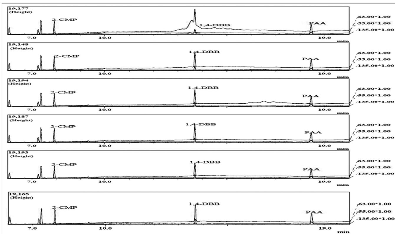
Fig. 9: Limit of quantification precision chromatograms for 2-chloro methyl propionate, 1,4-dibromo butane and para anisic aldehyde
