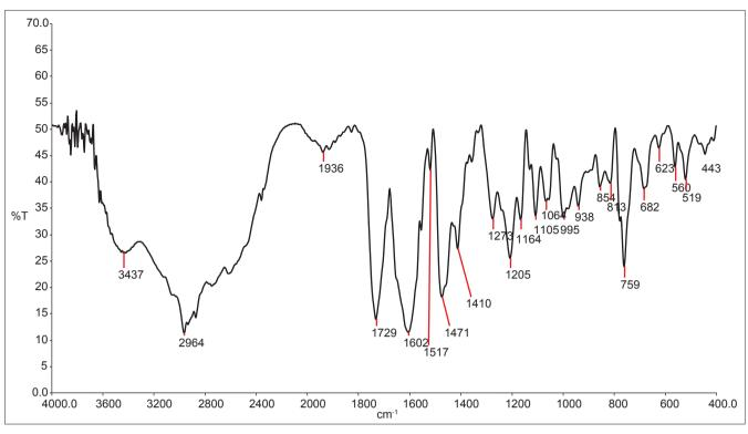
Fig.1: Infrared spectra of valsartan
