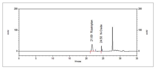
Fig. 6: Typical chromatogram of resolution solution of rizatriptan and N-oxide
