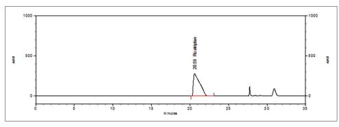
Fig. 5: Typical chromatogram of Id solution of rizatriptan
