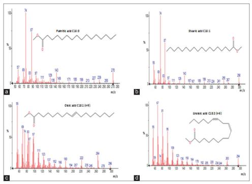
Fig. 2: (a-d) Mass spectrum of methyl esters fatty acids from tocte oil
