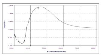
Fig. 1: Ultraviolet-visible spectrum of aqueous silver nitrate with aqueous extract of the seeds of *Anethum graveolens*
