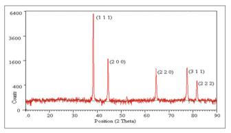
Fig. 2: X-ray diffraction pattern of silver nanoparticles synthesized using aqueous extract of the seeds of *Anethum graveolens*
