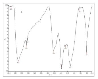
Fig. 3: Fourier transform infrared spectrum of silver nanoparticles synthesized using aqueous extract of the seeds of Anethum graveolens
