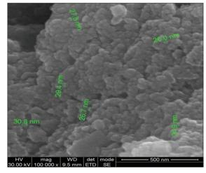
Fig. 4: Scanning electron microscopy micrograph of silver nanoparticles synthesized using aqueous extract of the seeds of *Anethum graveolens*
