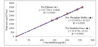
Fig. 6: Linearity curves of besifloxacin hydrochloride in diluent, in phosphate buffer, in simulated tear media
