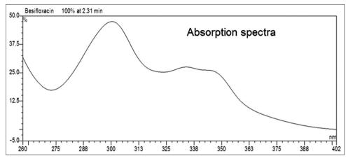
Fig. 2: Absorption spectrum of besifloxacin hydrochloride
