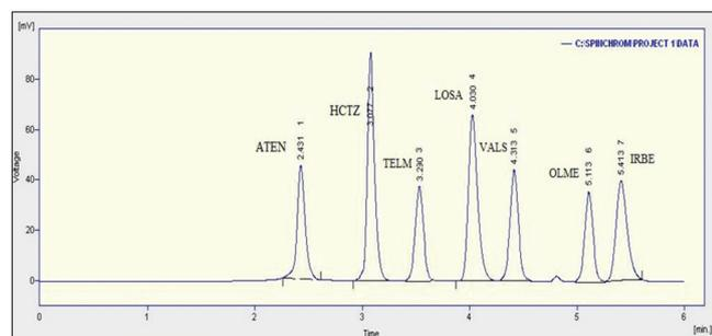
Fig. 1: A typical chromatogram showing the separation of atenolol and five angiotensin receptor blockade in the presence of hydrochlorothiazide mixture
