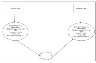
Nodes performing encryption and decryption function using random key.
