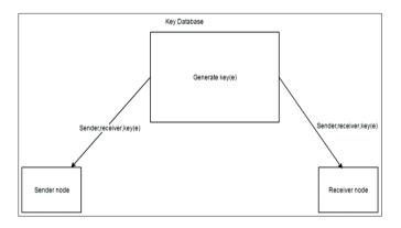
Key database generating random key and sending it to both sender and receiver node.
