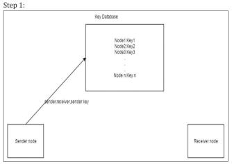
Sender requesting key database for random key by providing its key and receiver node id.
