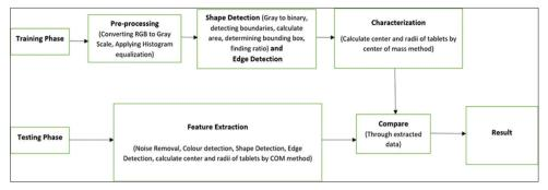
Fig. 1: Architectural diagram for characterization of pharmaceutical blisters
