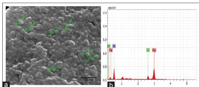
Fig. 2: (a) Scanning electron microscope micrograph of approach to synthesize silver nanoparticles and (b) corresponding energy dispersive X-ray spectrum
