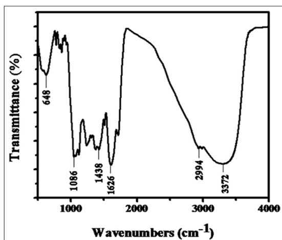
Fig. 3: Fourier transform infrared spectroscopy spectrum of silver nanoparticles
