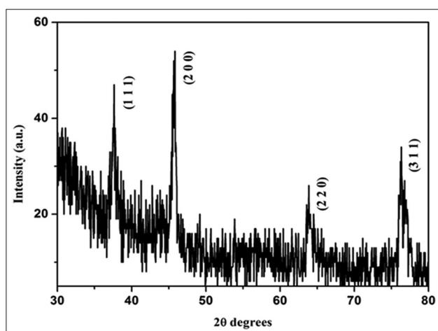
Fig. 4: X-ray diffraction pattern of approach to synthesize silver nanoparticles synthesized using *Nardostachys jatamansi* leaf extract
