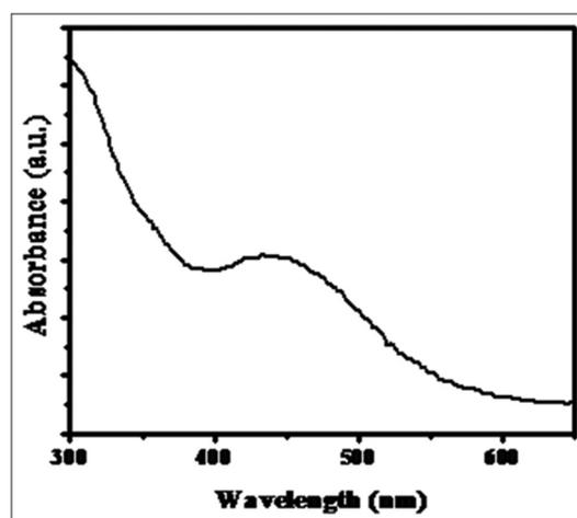
Fig. 1: Ultraviolet-visible spectrum of silver nanoparticles
