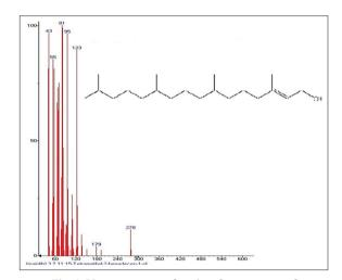
Fig. 4: Mass spectrum showing the presence of 3,7,11,15-Tetramethyl-2-hexadecen-1-ol
