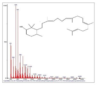
Fig. 14: Mass spectrum showing presence of 2,2,4-trimethyl-3-(3,8,12,16-tetramethyl-heptadeca-3,7,11,15-tetraenyl)cyclohexanol
