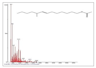
Fig. 2: Mass spectrum showing the presence of 10-methyl-8tetradecen-1-ol acetate
