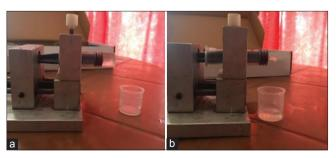
Fig. 9: (a) 5 ml syringe entirely filled with water before dispensing, (b) 2.5 ml of water dispensed into a measuring cap after running the device
