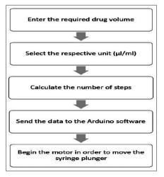
Fig. 7: Algorithm for the Android application
