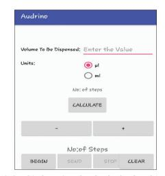
Fig. 8: Graphical user interface for the developed Android application
