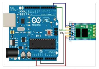
Fig. 5: HC-06 bluetooth module connections with Arduino integrated development environment software
