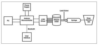
Fig. 2: Block diagram of the designed ocular drug delivery system
