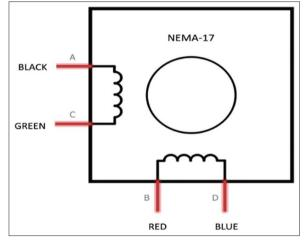
Fig. 4: Wiring schematic of NEMA 17 stepper motor
