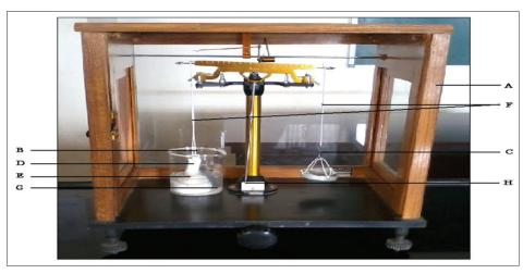
Fig. 3: *In vitro* bioadhesive strength measurement. (a) *In vitro* bioadhesive strength measurement modified balance apparatus, (b) left pan, (c) right pan, (d) teflon cylinder, (e) goat mucosa, (f) threads, (g) beaker containing solution, (h) pointer
