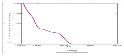
Fig. 11: Spectrum of S commercial tablet
