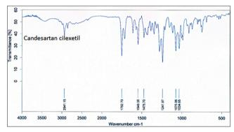
Fig. 1: Fourier transform infrared spectrum of candesartan cilexetil
