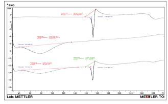
Fig. 6: Differential scanning calorimetry thermo grams of candesartan cilexetil (a), hydroxypropyl- $\beta$  cyclodextrin (b) and inclusion complexe1:1 (c)
