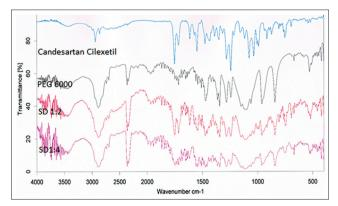
Fig. 2: Fourier transforms infrared spectra of candesartan cilexetil, solid dispersion 1:2 and solid dispersion 1:4
