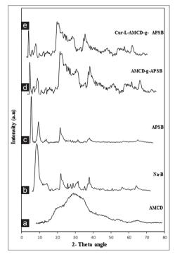
Fig. 3: X-ray diffraction of (a) acrylamide β-cyclodextrin (AMCD) (b) sodium bentonite (c) 3-aminopropyltriethoxysilane bentonite (APSB) (d) AMCD-grafted-APSB (AMCD-g-APSB) (e) curcumin-L-AMCD-g-APSB
