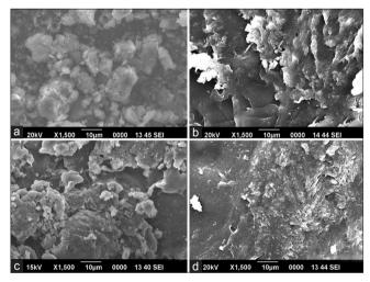
Fig. 5: Scanning electron microscope images of (a) grafted 3-aminopropyltriethoxysilane bentonite (APSB) (b) acrylamide β-cyclodextrin (AMCD) (c) AMCD-grafted-APSB (AMCD-gAPSB) and (d) curcumin-L-AMCD-g-APSB
