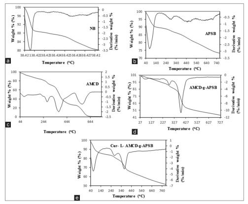
Fig. 4: Thermogravimetry-differential thermal analysis of (a) Sodium bentonite (b) 3-aminopropyltriethoxysilane bentonite (APSB) (c) acrylamide β-cyclodextrin (AMCD) (d) AMCD-grafted-APSB (AMCD-g-APSB), and (e) curcumin-L-AMCD-g-APSB
