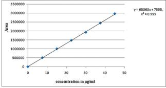
Fig. 5: Linearity graph of flurbiprofen
