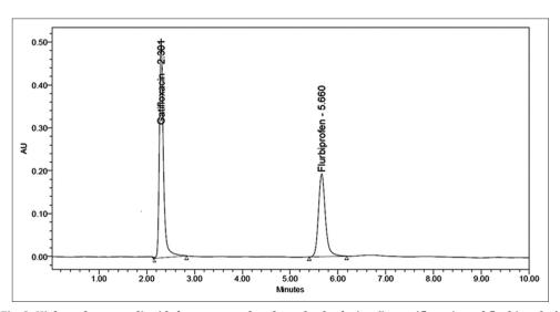
Fig. 3: High performance liquid chromatography of standard solution (i.e. gatifloxacin and flurbiprofen)
