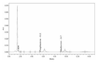
Figure 5: It shows HPLC-UV chromatogram of PIO and MET degradation in 30% H<sub>2</sub>O<sub>2</sub> (80°C).
