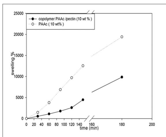
Fig. 4: Effect of time (minutes) onto the swelling percent of poly acrylic acid (PAAc) hydrogel and copolymer (PAAc/pectin) hydrogels at 30 wt% of AAC and 5 wt% of pectin and 20 kGy
