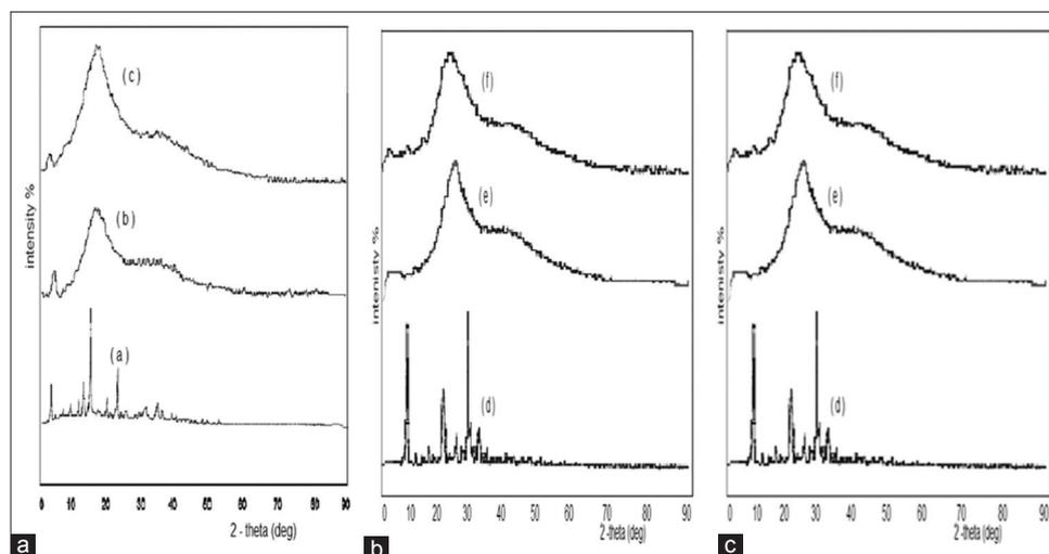
**Fig. 10: (A) X-ray diffraction (XRD) patterns of, (a) Pectin powder, (b) poly acrylic acid (PAAc) hydrogel and (c) copolymer (PAAc/pectin) hydrogels; (B) XRD patterns of, (d) drug ciprofloxacin, (e) PAAc hydrogel loading drug, (f) PAAc hydrogel release drug; (C) XRD patterns of, (g) copolymer (AAC/pectin) hydrogel loading drug, (k) copolymer (AAC/pectin) hydrogel release drug**
