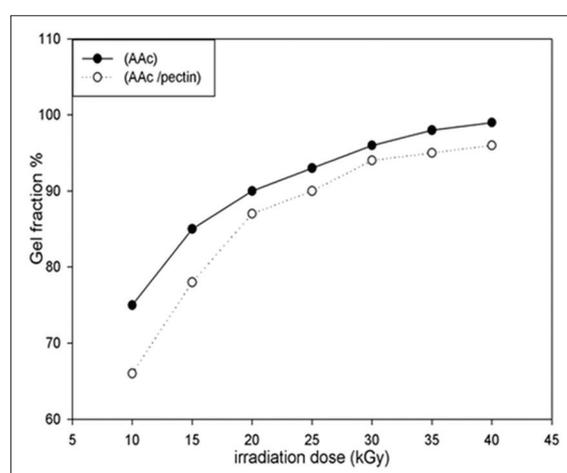
Fig. 3: Effect of different irradiation dose (kGy) onto the gel fraction percent of prepared (poly acrylic acid [PAAc]) hydrogel and copolymer (PAAc/pectin) hydrogels
