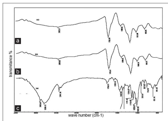
Fig. 9: Fourier-transform infrared spectrum of, (a) pectin powder, (b) poly acrylic acid (AAc) hydrogel, and (c) copolymer hydrogels (AAc/pectin)
