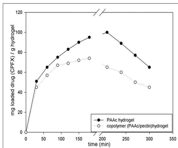
Fig. 6: The dependency of the drug loading amount to time (minutes) of (poly acrylic acid [PAAc]) hydrogel and copolymer (PAAc/pectin) hydrogels in pH 7
