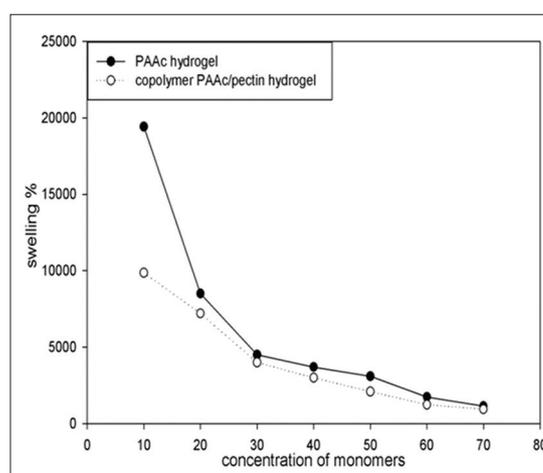
Fig. 2: Effect of monomer concentrations onto the swelling ratio after 24 hrs of (poly acrylic acid [PAAc]) and copolymer (PAAc/pectin) hydrogels
