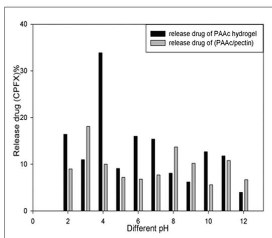
Fig. 7: Effect the different pH on the drug released of (poly acrylic acid [PAAc]) hydrogel and copolymer (PAAc/pectin) hydrogels after 24 hrs
