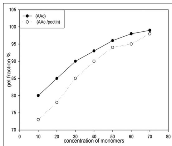
Fig. 1: Effect of monomer concentrations onto gel fraction percent of (poly acrylic acid [PAAc]) and copolymer (PAAc/pectin) hydrogel
