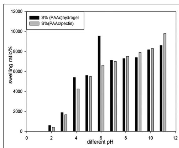
Fig. 5: Effect of different pH onto swelling percent of (poly acrylic acid [PAAc]) hydrogel and copolymer (PAAc/pectin) hydrogels after 24 hrs and 20 kGy
