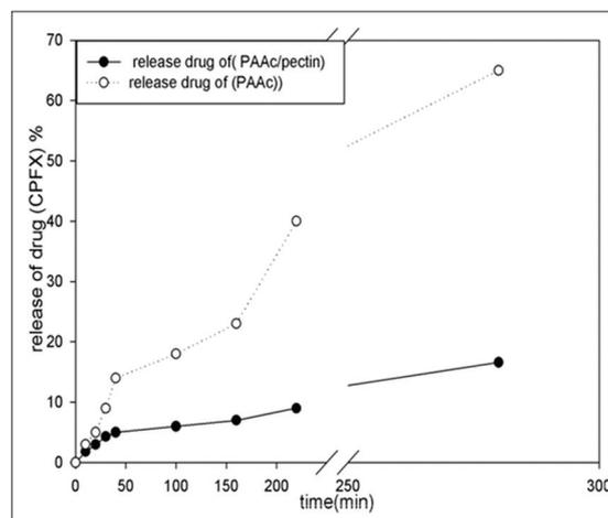
Fig. 8: Effect the drug release of (poly acrylic acid [PAAc]) hydrogel at pH 4 and copolymer (PAAc/pectin) hydrogels at pH 3 at different time (minutes) loaded with ciprofloxacin
