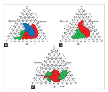
Fig. 1: Ternary phase diagrams, for avocado oil, sucrose esters (a) Laureate, (b) palmitate, (c) oleate and glycerin
