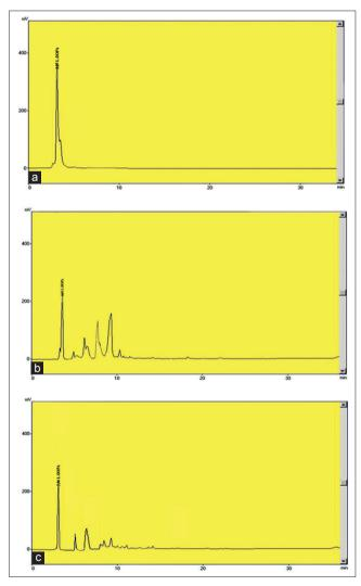
Fig. 3: High-performance liquid chromatography analysis of L-DOPA compound from *Mucuna pruriens* seed and callus extract (a) L-DOPA standard (1 mg/1 mL) - Sigma-Aldrich. (b) The seed extract of *M. pruriens*. (c) Callus extract of *M. pruriens*
