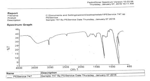
Fig. 9: FTIR of pure chitosan
