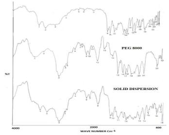
Fig. 2: FTIR spectra of drug DM, carrier PEG 8000 and solid dispersion of DM with PEG 8000
