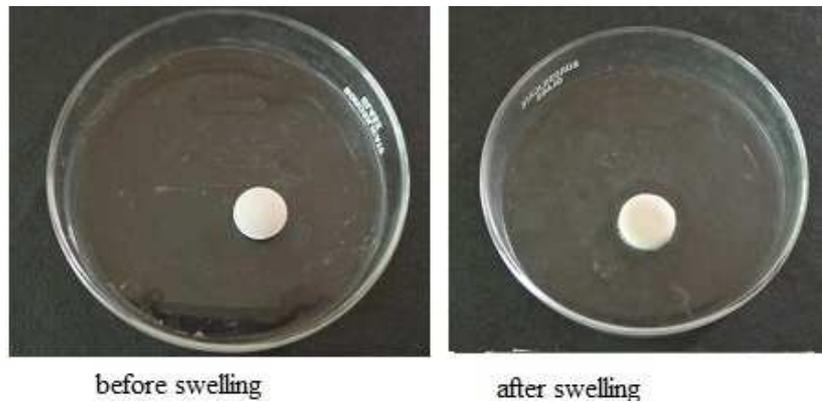
Fig. 7: Tablet image before and after swelling
